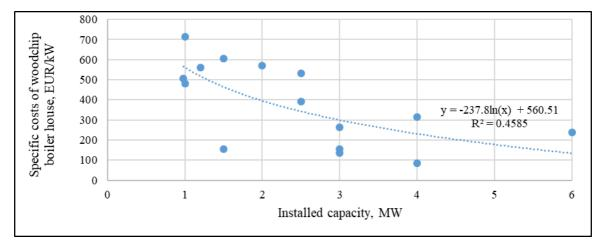
Fig. 3.1.29 Specific costs of woodchip boilers, materials and installation depending on boiler capacity
