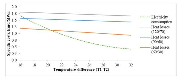
Fig. 2.1.4 Specific transmission cost dependence of supply and return water temperature difference
