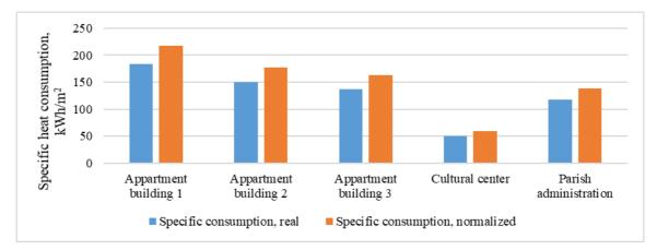
Fig. 3.2.8 Specific heat consumption of consumers (real and corrected)
