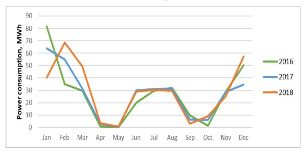
Fig.1 Electricity consumption of Nākotnes Street boiler house
