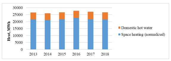
Fig.3.1.4 Normalized heat consumption for heating (blue) and hot water (red) production
