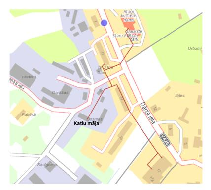
Fig. 3.2.5 The location of the heating pipes in the Stari village
