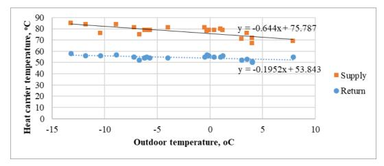
the obtained regression equations, a boiler house temperature curve is constructed (Fig. 3.1.6).
