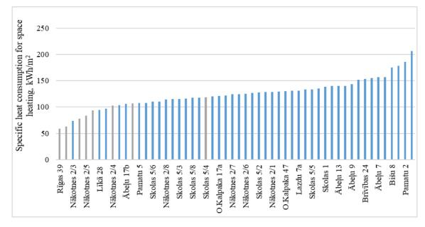
Fig. 3.1.11 Average specific heat consumption for heating in apartment buildings over the last 6 years. Renovated buildings are grey
