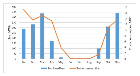
Fig. 3.5.4 Quantity of heat purchased in 2018, electricity consumed for heat transmission
