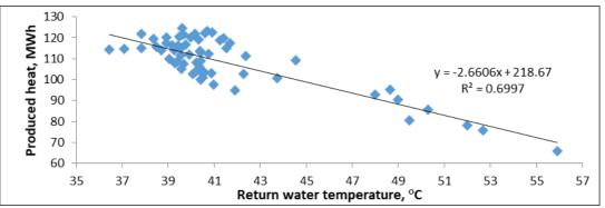
Fig. 3.1.14 Example of flue gas condenser operation depending on return temperature
