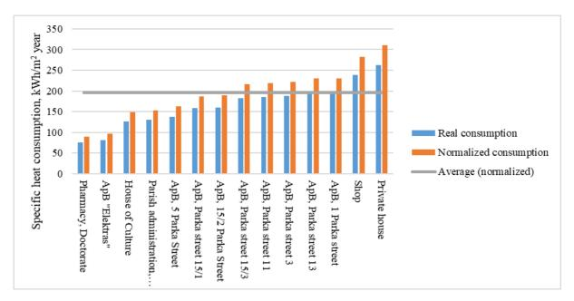
Fig. 3.5.2 Specific heat consumption (real and normalized) of DH connected buildings in Lizums
