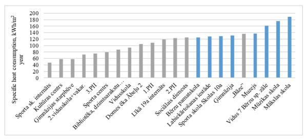
The specific heat consumption of municipality buildings for heating is given in Fig. 3.1.12.
