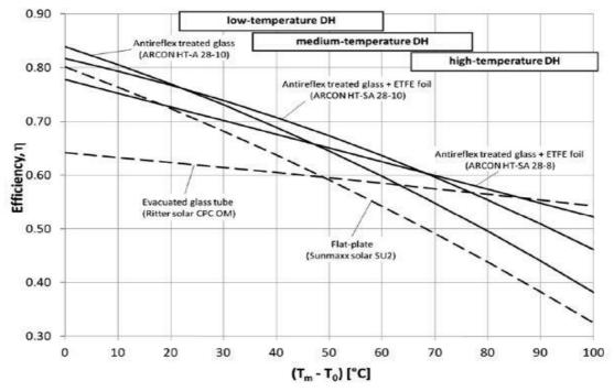
Fig. 2.2.6 Solar collector efficiency versus temperature difference between heat carrier and ambient temperature [27]
