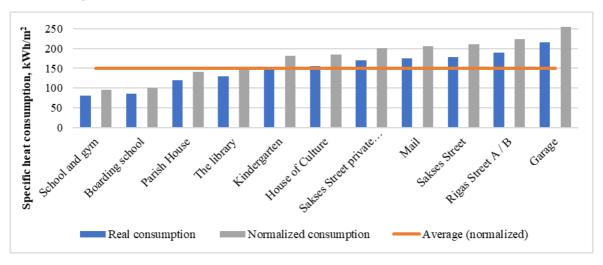
Fig. 3.4.4 Specific heat consumption for heating of DH connected buildings (actual consumption in the 2018/2019 heating season and normalized values)
