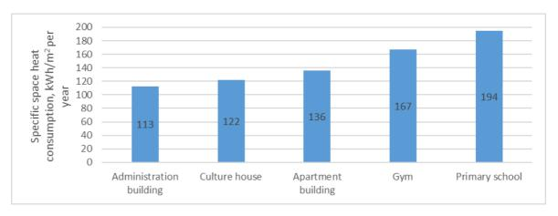
Figure 3.6.3. Specific heat consumption for space heating
