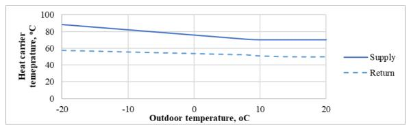
Fig. 3.1.6 Gulbene DH temperature curve
