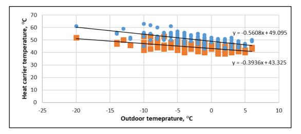
Fig. 3.2.3 Correlation of supply and return flow with outdoor air temperature
