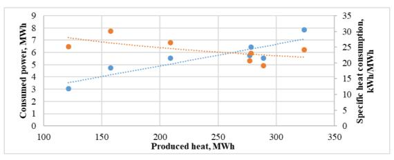
Fig. 3.4.8 Correlation of Electricity Consumption and Specific Electricity Consumption with the Heat Generated
