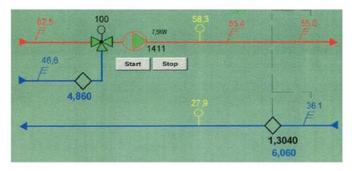
Fig. 3.1.18 Example of a technological solution for a three-stream mixing plant [41]
