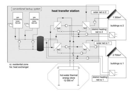
Fig. 2.4.5 Hydraulic diagram of integrated solar heating system in Friedrichshafen [51]
