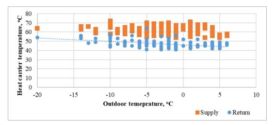
Fig. 3.4.6 Correlation of flow and return flow with outdoor air temperature
