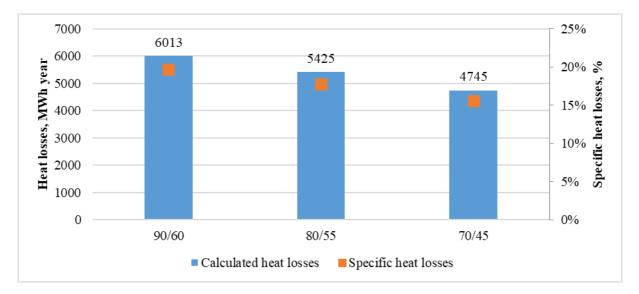
Fig. 3.1.15 Modeled heat losses and specific heat losses at different temperature graphs
