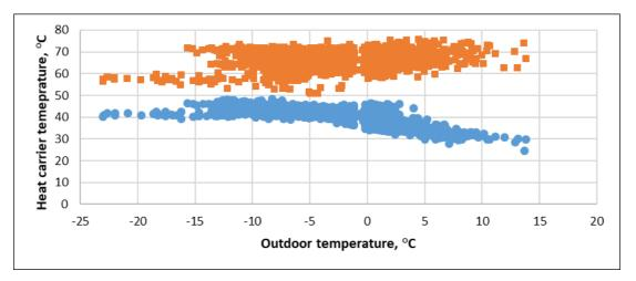
Fig. 5.1.2 Correlation between heat carrier temperature and outdoor air temperature
