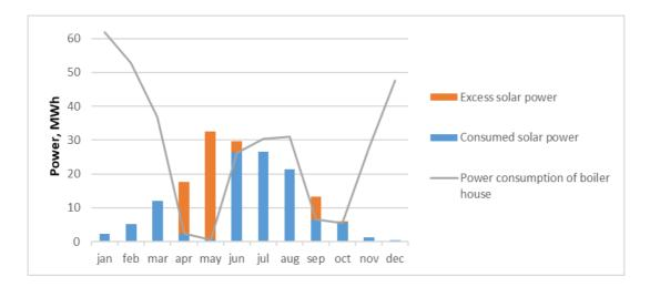
Fig. 2 Average Electricity Consumption Boiler House (green line), Solar Electricity Consumption (blue) and surplus solar power (red)
