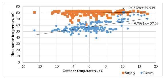
Fig. 3.5.5 Correlation of flow and return flow with outdoor air temperature
