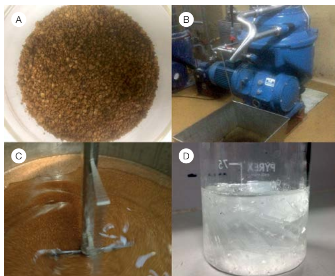
A: Recovered raw cellulose. B: Centrifugation to separate stone and ionic liquid. C: Ionic liquid and stone. D: Ionic liquid. Photos: Operational Group.
