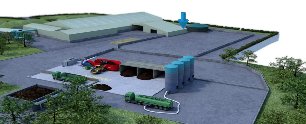
Feed from Solid Feeding System & Liquid Storage Tanks to Primary Digesters, then to After Digester
