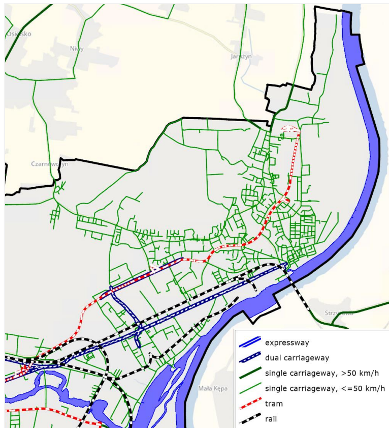
Figure 5. Bydgoszcz transport model – overview of road network in eastern (Fordon) area.
