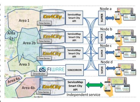
redirect the queries to the nodes that could provide the service and data. Thus, the **Supers** do not need to hold the data of the nodes and perform the distribution of queries only to the involved nodes, to finally collect the results and performs data fusion. The **Supers as well as the ServiceMaps** may also implement some query caching solution as all the other **Federated Knowledge Bases**.
