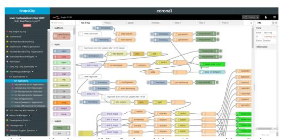
Snap4City platform provides a large set of **MicroServices**, which provide an easy and formalized access to all the Smart City services that are available on-cloud from the platform (including the ones to control a part of the platform itself). They are made available in the Node-RED Node.JS environment to create **IoT App** as visual programming language. Among the **MicroServices**, the **IoT Apps** also need to access such services to allow for
