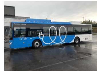
2019 -> Yutong depot-charged (300 kWh)
