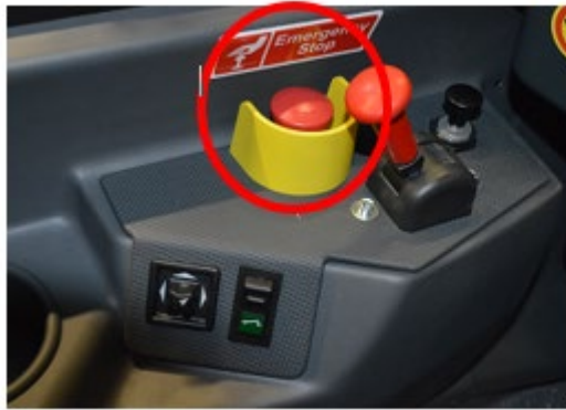
Emergency stop switches
