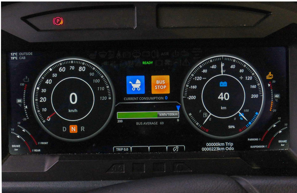
Electronic instrument cluster of an electric bus. Photo by Markku Ikonen.
