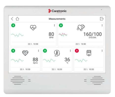
**Automatic wireless transmission** of **vital signs measuremenets** to the HomeTab device enables continous **monitoring** and gives **alert** to the caregivers when a value requires immediate attention.
