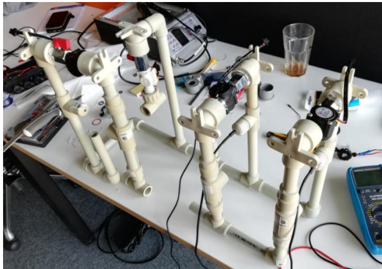
Figure 22 Cybercom's PoC of the system for online water quality monitoring and E. coli detection
