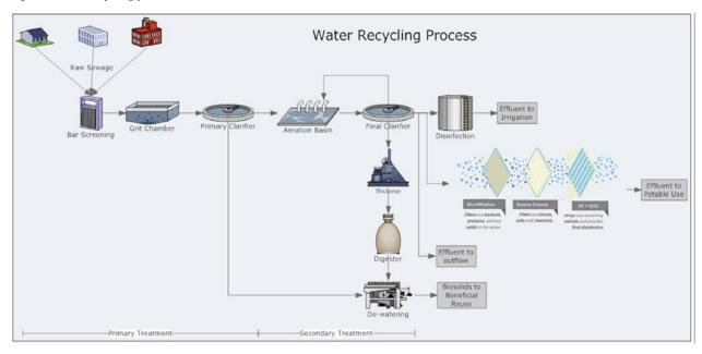
Primary sedimentation follows, eliminating most of the suspended materials and, if some of these solids are biodegradable, the biochemical oxygen demand (BOD) is typically reduced. Then, secondary treatment usually involves a biological process. Microorganisms in suspension (in the "activated sludge" process), are used to remove biodegradable organic material.
